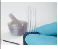
Sample preparation can be time-consuming. Our innovative sample preparation tool holds up to six samples and simplifies the correct filling process. Its unique design allows you to insert the capillaries directly into the instrument.
