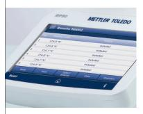
Perform different measurements quickly and efficiently by working with up to 60 methods. Results are displayed immediately after the experiment, and up to 100 results are stored automatically and can be accessed at any time directly on the instrument.
